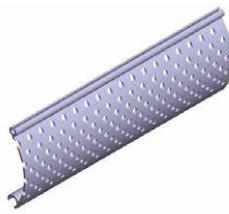
PERFORATED Resistance class: 3 EN 1627 Slat weight: 6,2 kg/m 2 Opening ratio: 25,3 % Opening size: ø 4 mm
